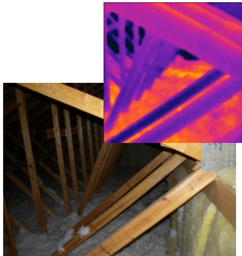
Area over master bathroom showing effect of unboxed bathroom fan
